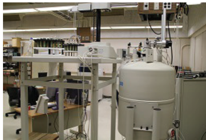
Varian Inova 300 with automatic sample changer (VI-300)
