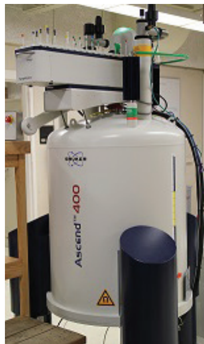
Bruker Avance III HD with SampleXpress (AX-400)
