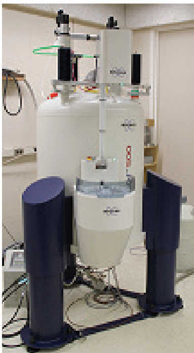
Bruker Avance III 500 with SampleCase (AV-500)
